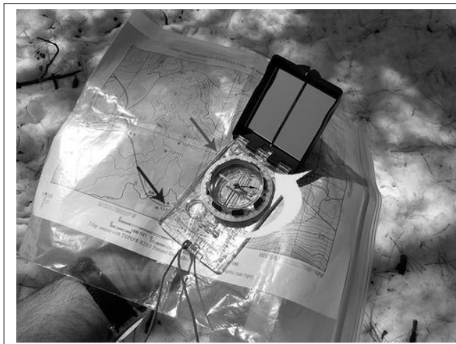
Figure 9.31. Taking azimuth from map
