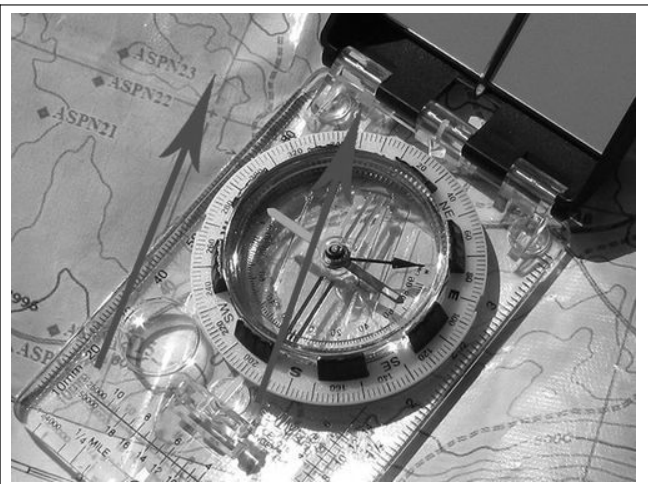
Figure 9.32. Orienting lines parallel to map NS lines
