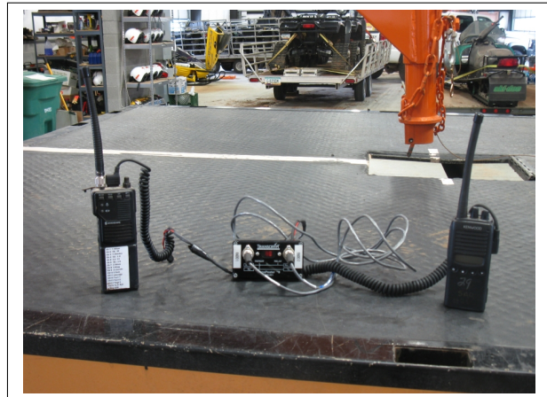
Figure 17.2. A portable repeater using two hand-held radios
