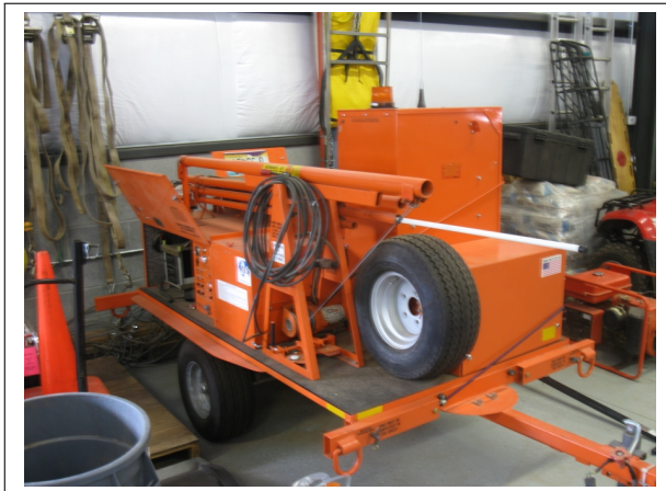
Figure 17.1. A trailer-mounted portable repeater unit
